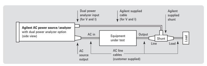
Test configuration of efficiency measurement using an Agilent AC power source/analyzer with the 020 dual power analyzer option.
